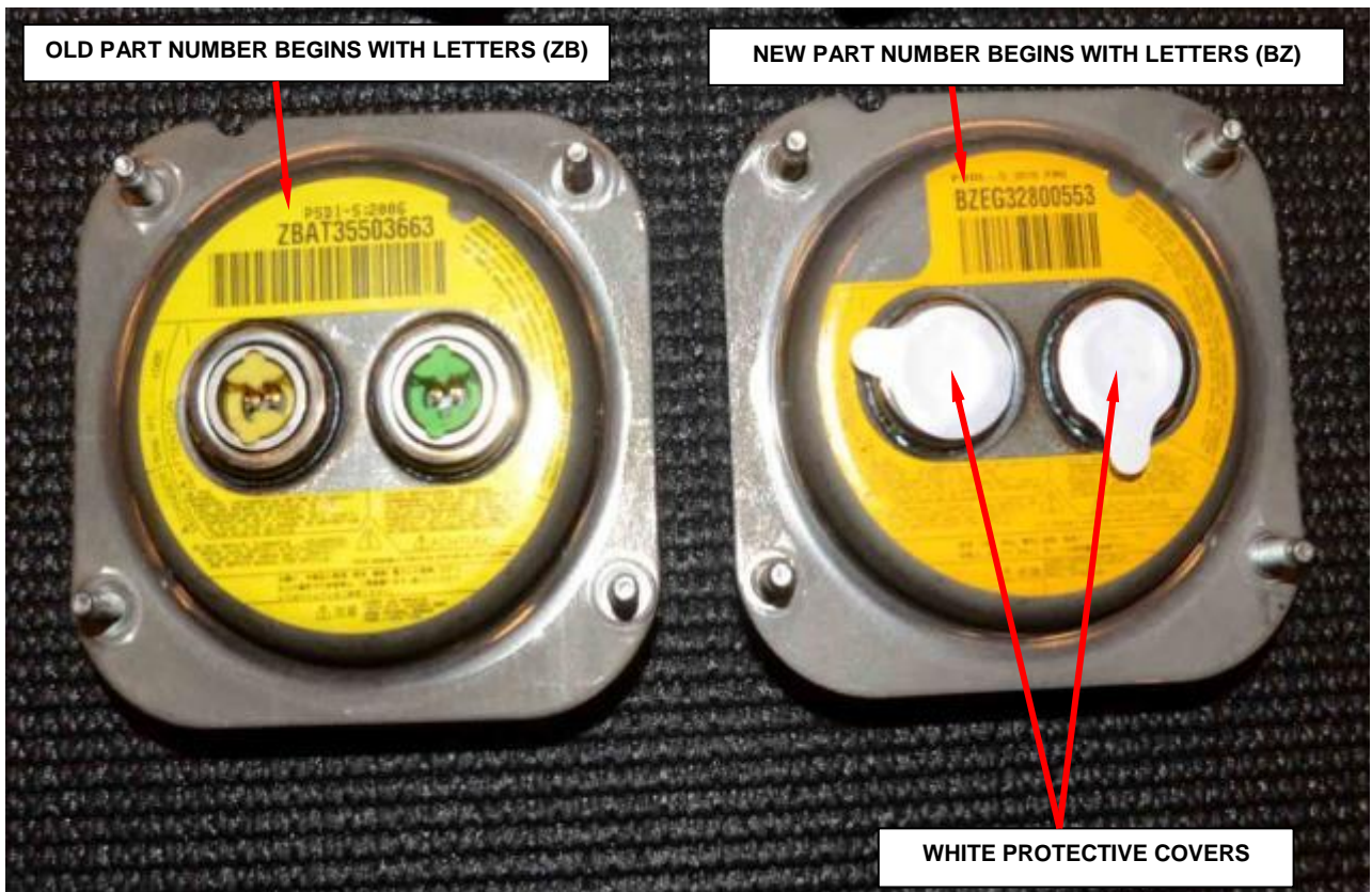
Figure 11 – Driver Airbag Inflator
