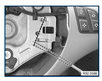
Insert Torx screwdriver (T25) at an angle into concealed opening on reverse side of steering wheel until a spring resistance is felt (approx. 1.5 cm).
