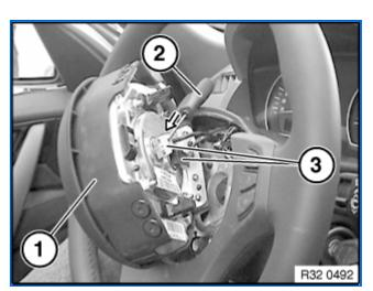
Tilt airbag unit (1) slightly to one side. Slide screwdriver (2) from front into both plug connections (3) until cover lifts off.
