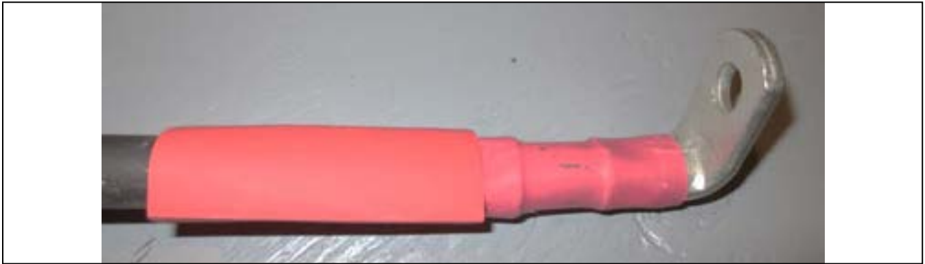
Figure 5 - Positioning of the 2.5 Inch Red Shrink Tubing on the Cable and Connector
