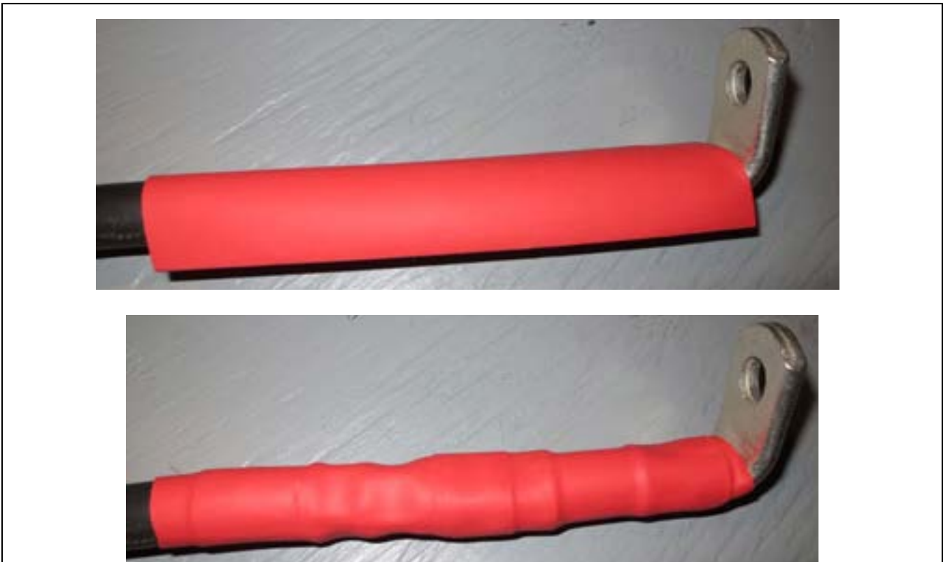
Figure 6 - 5 Inch Red Shrink Tubing Positioned and Properly Shrunk
