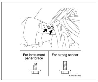
c) Using the 2 bolts, attach the lower part of the instrument panel brace No. 1.
