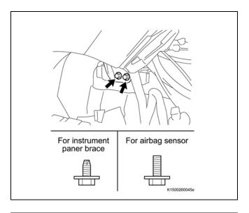
c) Remove the 2 bolts from the bottom part of the instrument panel brace No. 1.
