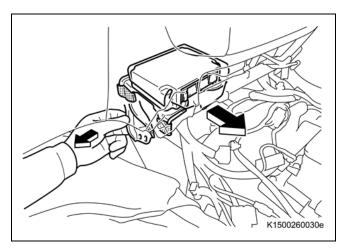
e) While pulling the instrument panel brace No. 1, slide the center airbag sensor assembly to the rear of the vehicle and remove it.
