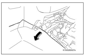
a) Pull the floor carpet back from the lower part of the instrument panel.
