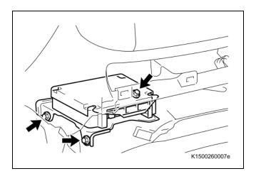
d) Remove the protective tape, and then use the 3 bolts to install the center airbag sensor.
