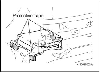
d) To prevent floor damage, apply protective tape to the brackets of the center airbag sensor in the locations shown in the illustration.
