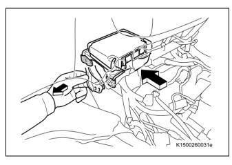
b) While pulling the instrument panel brace No. 1, slide the center airbag sensor into place.
