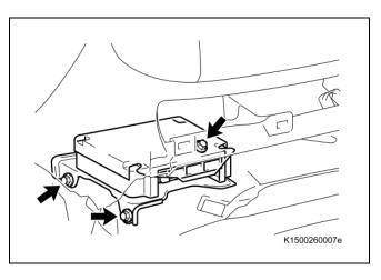
b) Remove the 3 bolts from the center airbag sensor.
