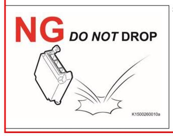
3. DO NOT DROP THE CENTER AIRBAG SENSOR
