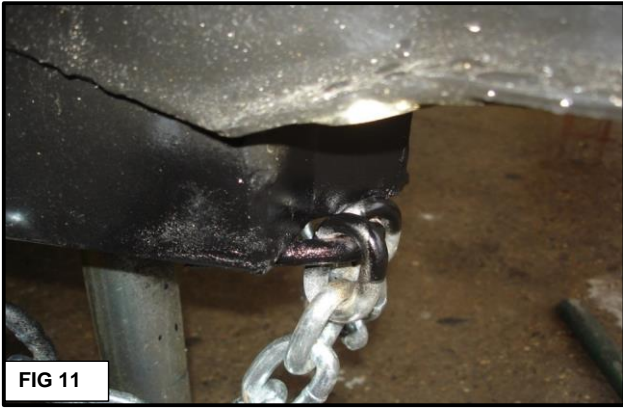
Fig 11: Let welds cool then paint it black with a good quality spray paint (like Rustoleum) Chains should move freely on the chain elbow(s).
