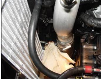
6. Use pliers to release the clamps (D) of both oil cooler hoses (Yellow and Red) on the transaxle side.
