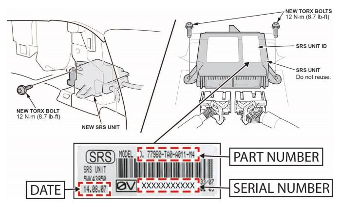
7. Connect the SRS connectors to the SRS unit by pushing the connector in and the lever moves to the locked position.
