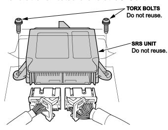
6. Write down the new SRS unit ID (serial number) on the RO, then install the new SRS unit using the new Torx bolts. NOTE: Make sure the SRS unit is sitting squarely against its bracket before torqueing the Torx bolts.
