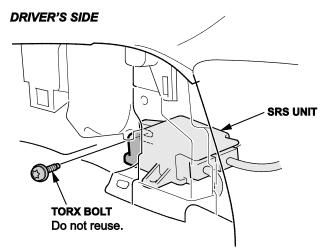
4. Disconnect the SRS unit connectors from the SRS unit by releasing the lever locks, then pull on the lever to disconnect the connectors.
