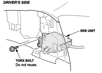
4. Disconnect the SRS unit connectors from the SRS unit by releasing the lever locks, then pull on the lever to disconnect the connectors.
