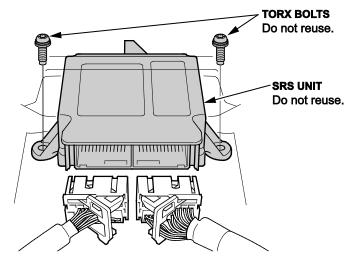
6. Write down the new SRS unit ID (serial number) on the RO, then install the new SRS unit using the new Torx bolts. NOTE: Make sure the SRS unit is sitting squarely against its bracket before torqueing the Torx bolts.
