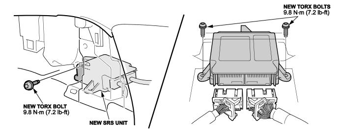
8. Connect the SRS connectors to the SRS unit by pushing the connector in and the lever moves to the locked position.
