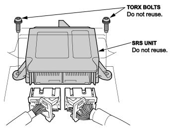
7. Write down the SRS unit ID (serial number) on the RO, then install the new SRS unit using the new Torx bolts.
