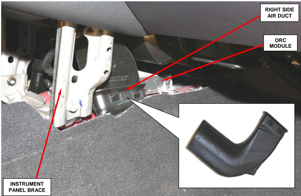
Figure 9 – Right Side Air Duct
