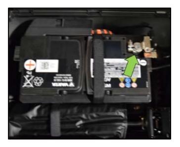
• Disconnect and isolate the negative battery cable <arrow>.
