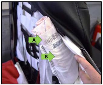
Install the replacement side airbag <arrow A> into the sewn in pocket in the seat cover <arrow B>.
