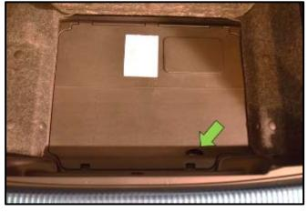
Install the battery access cover <arrow>.
