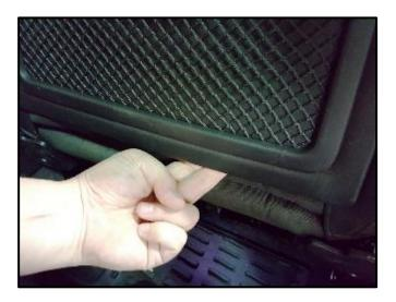
Locate the seat backrest cover hooks by hand <as shown>.
