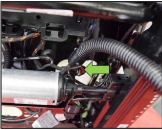
Install the retainer securing the wiring harness to the seat frame <arrow>.
