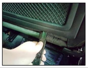
Once the hooks are located, insert pry lever 80-200 (or equivalent) underneath the hooks <as shown>.
