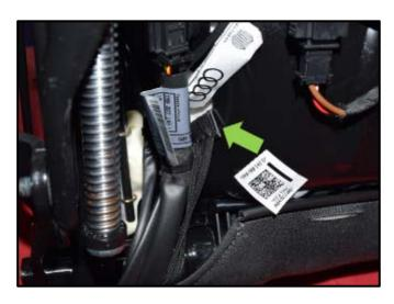
• On the underside of the seat, attach the outboard side retaining strap <arrow> to the seat bottom pan.
