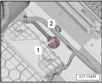
Remove nut <1> at ground connection, and remove ground cable <2> for the Battery.
