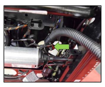
• Release the retainer securing the wiring harness to the seat frame <arrow>.
