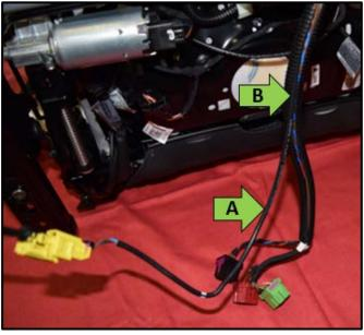
Remove the airbag wiring harness <arrow A>
