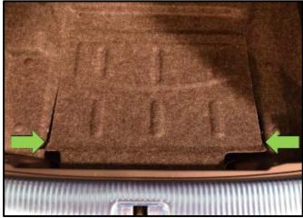
• Open the rear carpet cutaway <arrows>.
