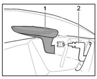
• If equipped, install the adjustment handle <1> to the adjusting lever <2>.
