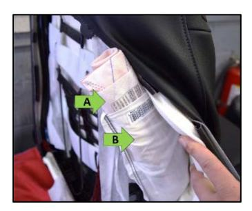
• Remove the side airbag <arrow A> from the sewn in pocket in the seat cover <arrow B>.
