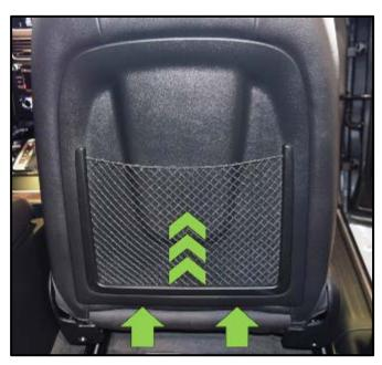
Release the lower seat backrest cover hooks by lifting up on the cover in the direction shown <directional arrows> and gently prying the seat hooks <arrows> up and towards the rear of the vehicle using pry lever 80-200 (or equivalent).
