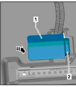
Reattach the front cover <1> connector station under the seat <2>.
