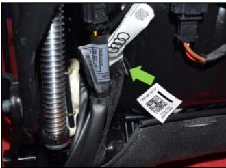
On the underside of the seat, release the outboard side retaining strap <arrow> from the seat bottom pan.
