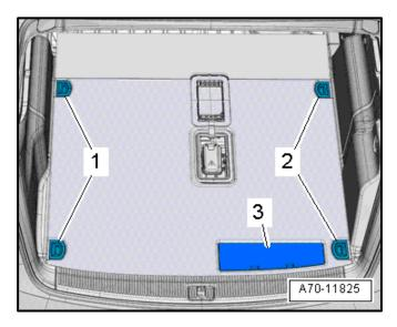
• Lift up and remove the luggage compartment floor panel and tool box <3> towards the rear.
