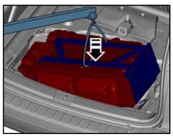
Using the retaining strap T40155 and the Shop Crane VAS6100 (or equivalent), lift the Hybrid Battery Unit (AX1) back into the vehicle and align it with the battery tray compartment.
