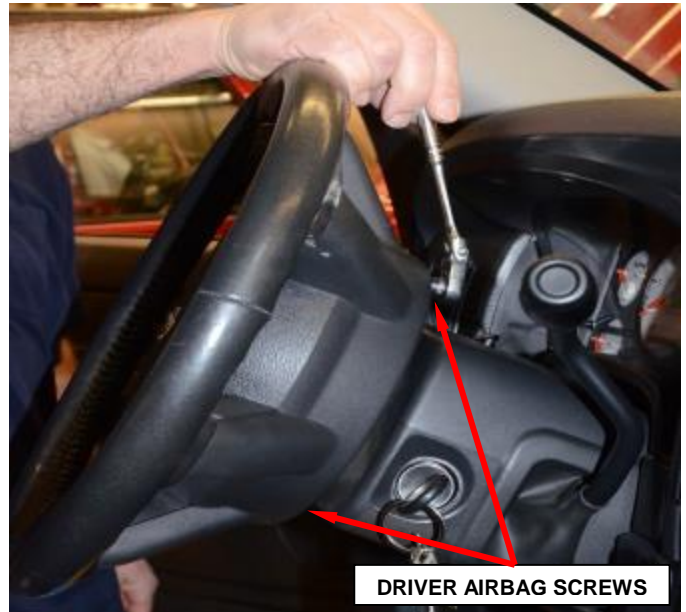
Figure 1 - Driver Airbag Screw Location
