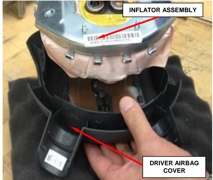
Figure 9 - Inflator Assembly to Driver Airbag Cover
