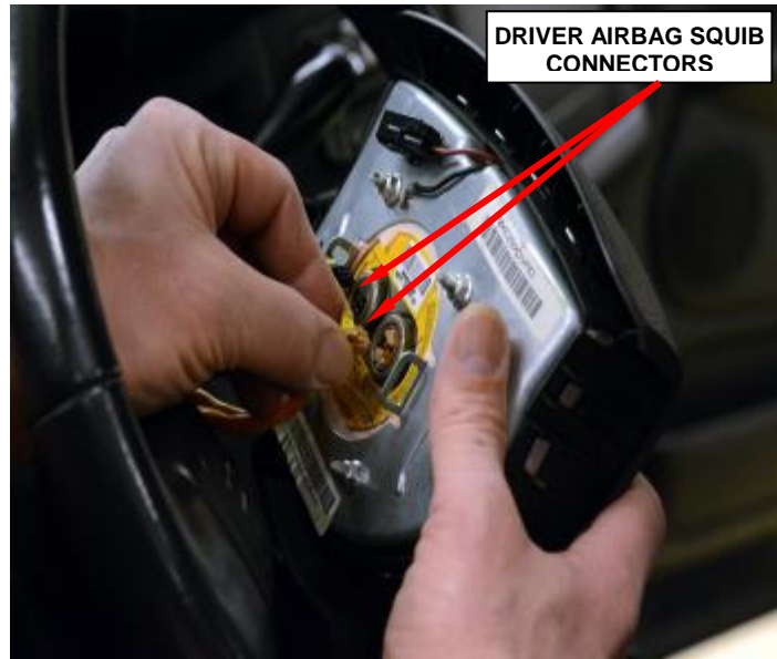
Figure 3 – Driver Airbag Squib Connectors
