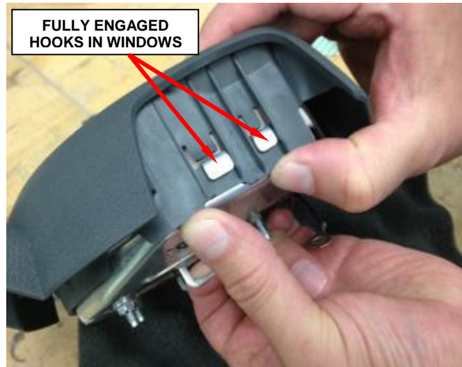
Figure 11 – Inflator Assembly Hooks
