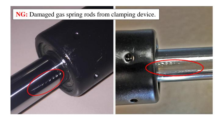
Always properly support the lift gate prior to removal of the old lift gate gas springs. **Do NOT take any shortcut by clamping the lift gate gas springs.**
