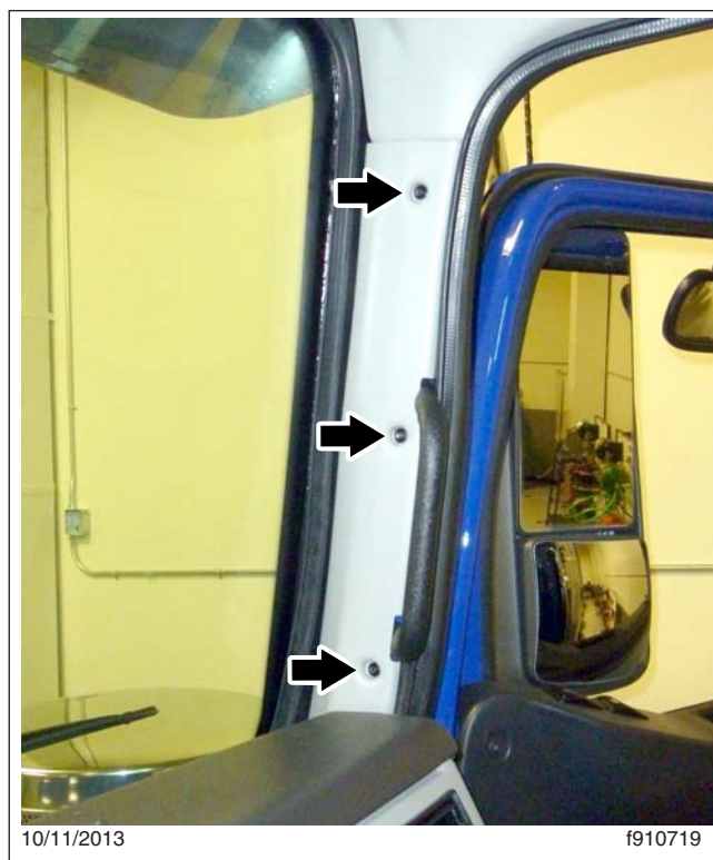
Fig. 3, A-Pillar Cover Screws
