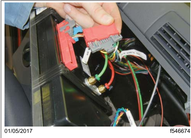
Fig. 14, ICU 2A connector Terminal Locks
