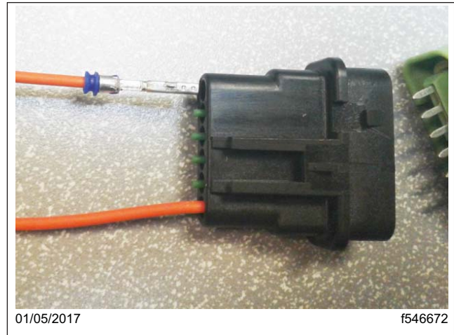
Fig. 12, Splice Pack Terminal Insertion
