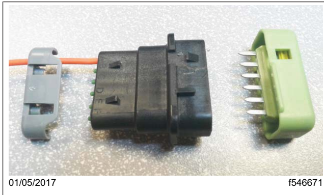
Fig. 11, Splice Pack Cover and Lock (removed)
