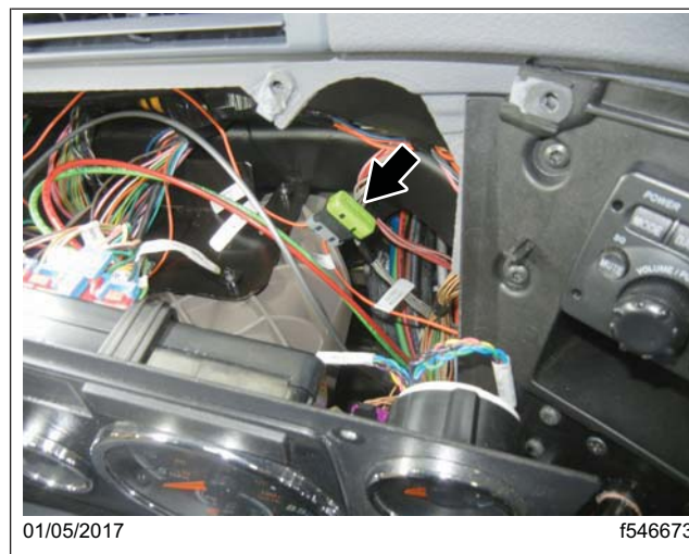
Fig. 13, Splice Pack Routing
