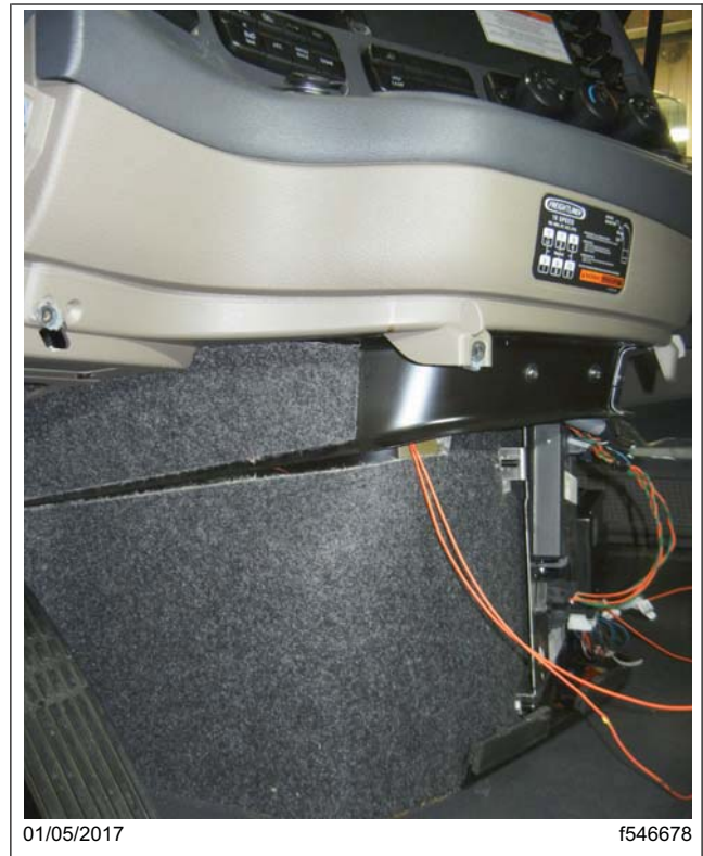
Fig. 18, Routing the Wires to the ABS Module (FL721-A installation shown)
