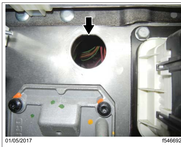
Fig. 33, Bulkhead Connector 1A Cavity on the Frontwall
