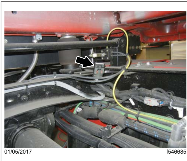
Fig. 25, CPDM Harness Capped
