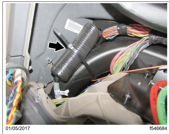
Fig. 24, PLC Bundle Mounting
