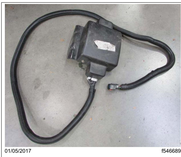
Fig. 29, CPDM Removed from the Vehicle
