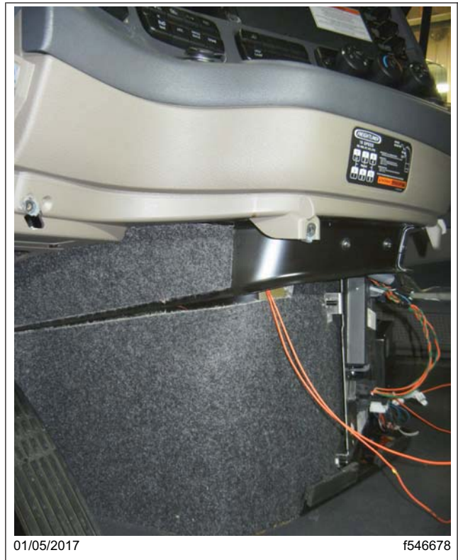
01/05/2017 f546678 Fig. 18, Routing the Wires to the ABS Module (FL721-A installation shown)
