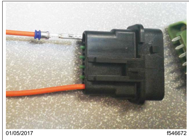
Fig. 12, Splice Pack Terminal Insertion
