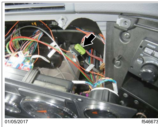
Fig. 13, Splice Pack Routing
