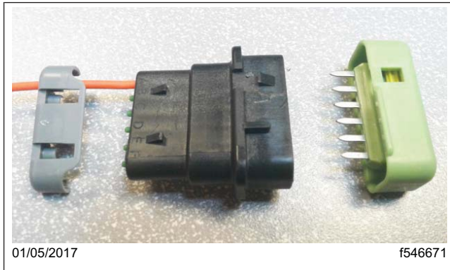
Fig. 11, Splice Pack Cover and Lock (removed)
