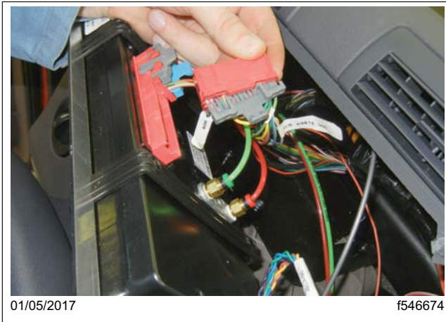
Fig. 14, ICU 2A connector Terminal Locks
