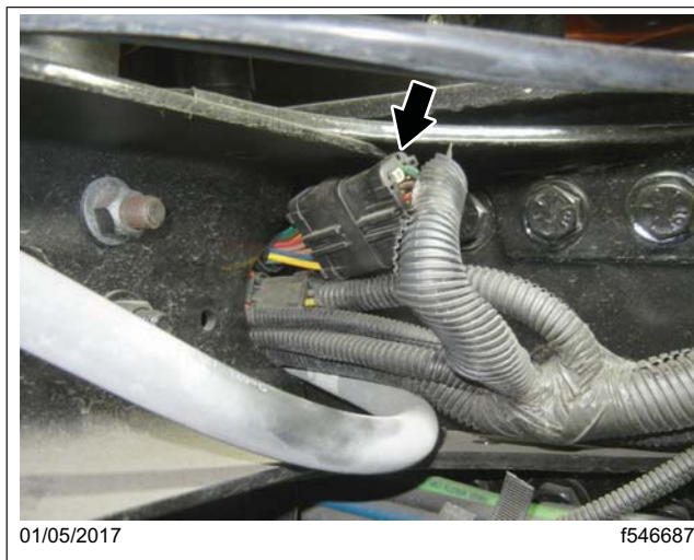
Fig. 27, CPDM Harness Connector
