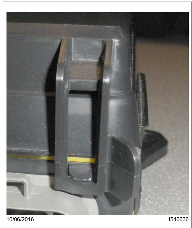
Fig. 2, Correct: Latch Cover Intact
