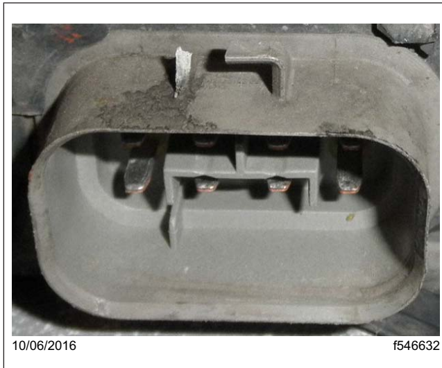
Fig. 3, Incorrect: Broken connector locking tab
