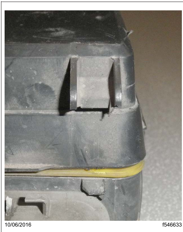
Fig. 1, Incorrect: Broken Latch Cover
