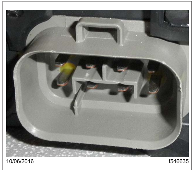
Fig. 4, Correct: Connector locking tab intact
