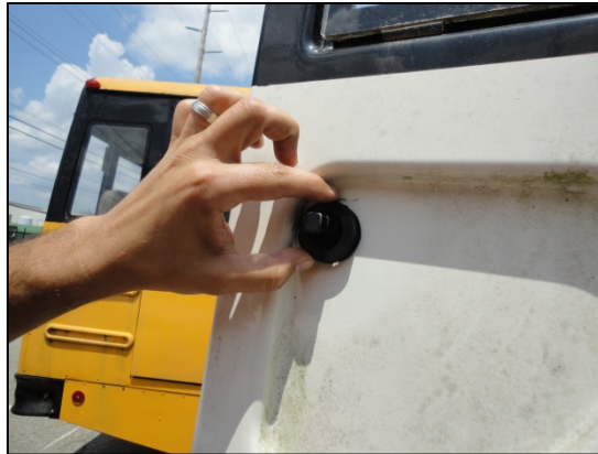
Figure 10, Installing the New Washer
