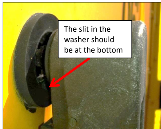
Figure 5, Position of Slit in Washer
