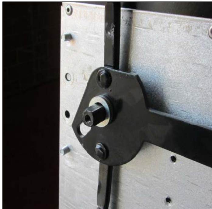
Figure 17, Handle and Shaft Mechanism Without the Latch Assembly
