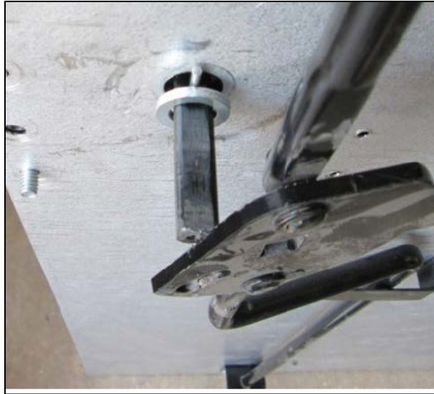
Figure 20, Inserted Pin and Washer
