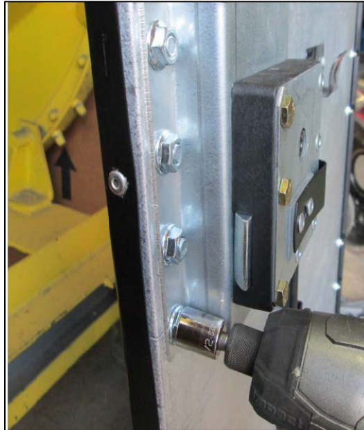
Figure 16, Removing 4 Nuts from the Door
