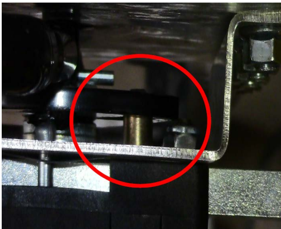
Figure 22, Guide Bushing Inserted in the Handle Slot
