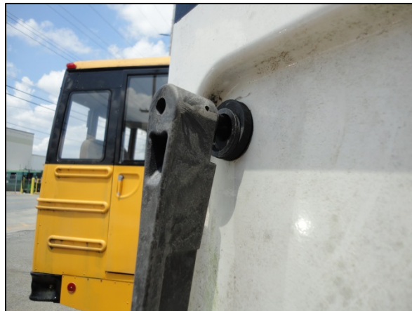
Figure 11, Position of Newly Installed Exterior Handle
