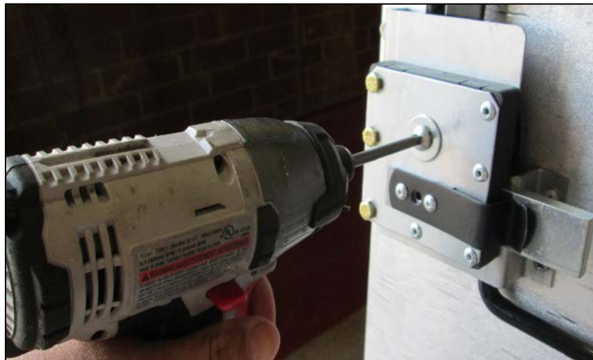
Figure 15, Removing the Bolt and Washers from the End of the Shaft
