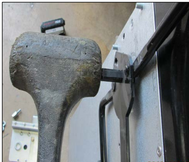
Figure 19, Tapping Out the Stem
