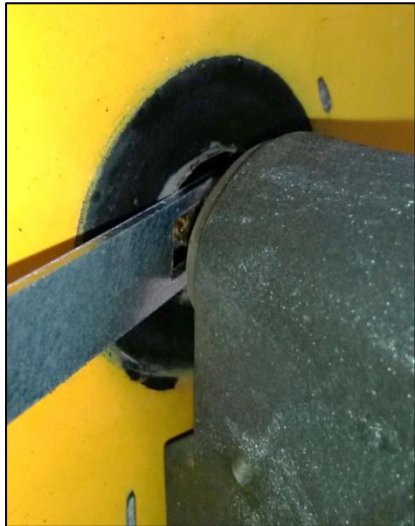
Figure 3, Using the Go/No Go Gauge
