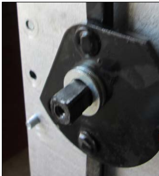
Figure 21, Handle and Rod Assembly on the Door Handle Stem
