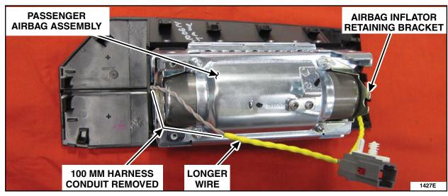
5. Position the shorting clip onto the harness wires, and crimp the shorting clip together one side at a time using pliers. See Figure 3.
