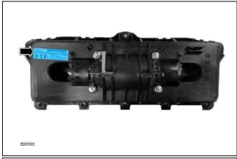
2. Locate the QR code on the NEW passenger airbag module label.
