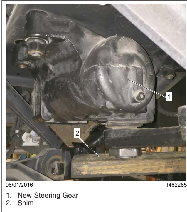
Fig. 14, New Steering Gear Installation
