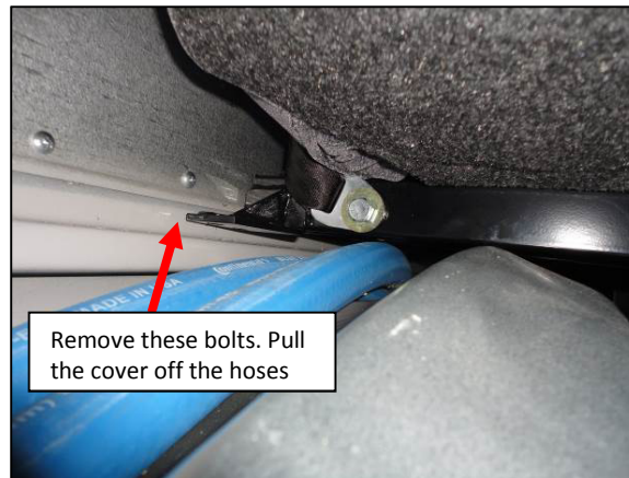
Figure 5, Remove Seat Rail Bolts to Remove Wheel Well Cover
