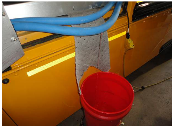
Figure 4, Drain Coolant From the Side Emergency Door Hoses
