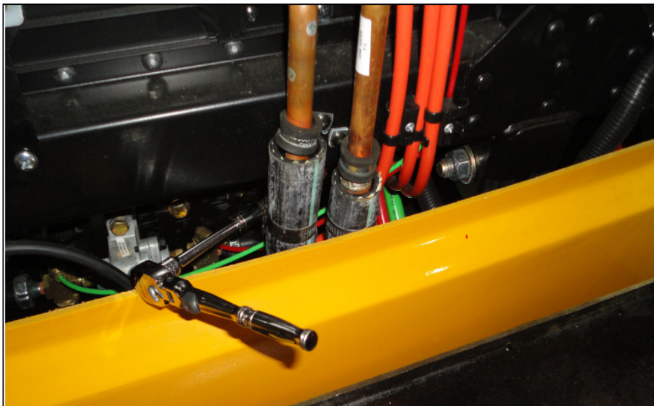
Figure 8, Front Firewall, Hoses Connect to Tubes as Shown
