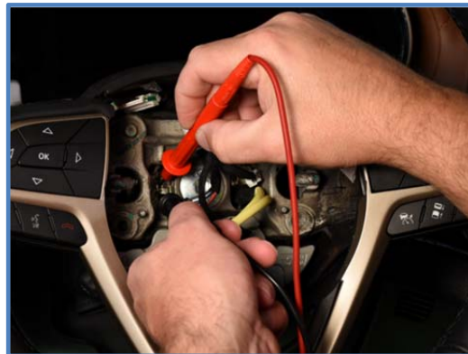
Figure 6: Testing terminal connection at the SCCM.
