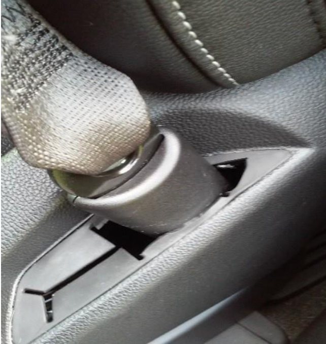
Example of poorly executed on-vehicle repair.
