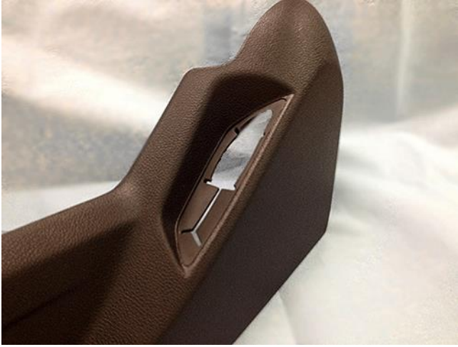
Example of properly executed repair before the seatbelt panel has been reinstalled on the vehicle.
