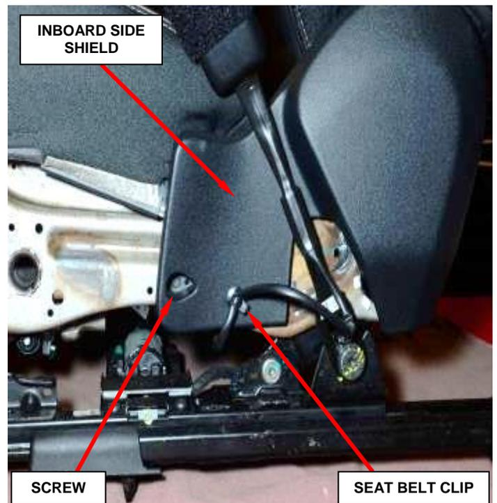
**Figure 6 – Inboard Side Shield**
