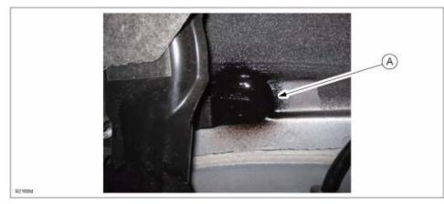
8. Reinstall the nut (A) onto the bracket. Verify the tightening torque shown below. Tightening Torque: 8.8 - 12.7 Nm {78 - 112 in-lbf, 89.7 - 129 kfg-cm}
