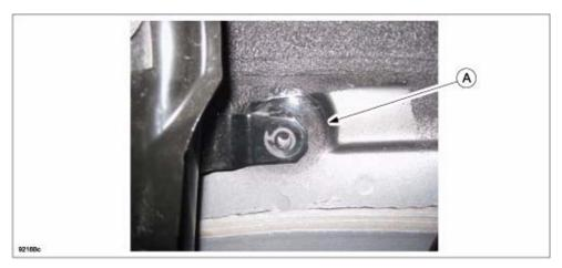
8. Spray the area (A) with a coat of VALUGARD undercoating.
