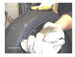
Measure 8-12 inches along the sidewall of the tire and then make a visible cut through sidewall of the tire that length. This method is described in the two photos above. Please use gloves and precaution when making the cut.
