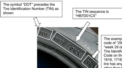
The example shows a date code of "2916", indicating "week 29 of 2016". The Tire Identification Date Code on the recalled tires is 1616, 1716 or 1816. If the tire has any Date Code other than the 3 listed above or is not a 180/55ZR17 M/C (73W) Pilot Power 3 tire, it is NOT affected by this Recall notice.
