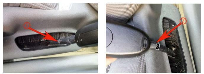
This inspection must be performed on both the driver and passenger side safety belt cable sleeve. If these front sleeves are cut or cracked either on the cable (see arrow 1 above) or where the cable meets the buckle (see arrow 2 above), the safety belt assembly should be replaced. If the sleeve shows only scuffs or wear marks (no cuts or cracks), replacement is not necessary.
