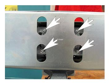
3. Position the air bag so that all four stopper plate nuts can be removed through the access holes.
