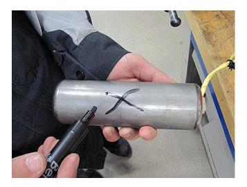
12. Put a mark on the removed inflator and store it in the provided replacement part box. Refer to the packaging instructions that were included with the new inflator module kit.
