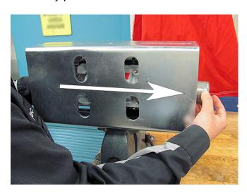
11. Remove the inflator from the housing, slide the inflator away from the harness side.
