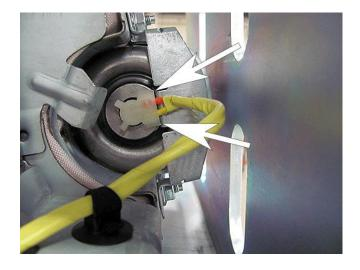
6. Note the orientation between the inflator and the stopper plate.
