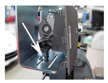
2. Using the hardware kit supplied with the module bracket, loosely mount the airbag assembly to the bracket using two nuts and bolts.
