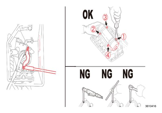
19. Tighten four (4) *NEW* plate nuts evenly in several increments in the order shown in the illustration using a 10 mm socket driver while pushing the inflator. You will encounter some resistance during tightening because these nuts are self-locking nuts. **Torque Specification:** 3.9 Nm (35 in-lb)
