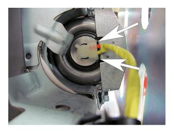
18. Rotate the inflator until the harness connector aligns with the Position Orientating Plate.
