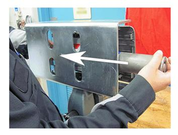
14. Carefully slide the new inflator into the air bag assembly. Ensure the inflator is installed with the harness end first.
