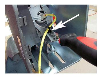
9. Disengage the wire harness locator from the housing.
