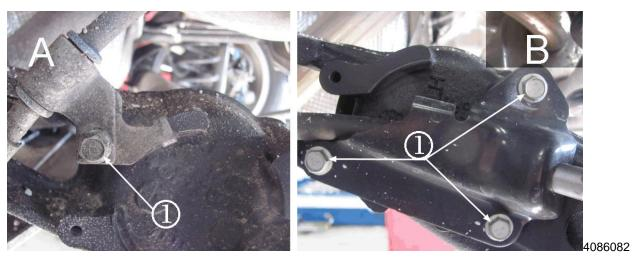
(A) Location of rear park brake cable bracket bolt (1) for vehicles equipped with disc brakes.(B) Location of rear park brake cable bracket bolts (1) for vehicles equipped with drum brakes.
