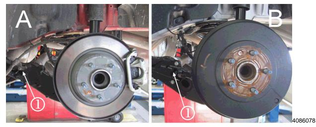
(A) Vehicles equipped with disc brakes. (B) Vehicles equipped with drum brakes.
