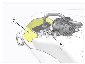
13. Torque the fuel pump screws in a star pattern following the specified torque sequence.
