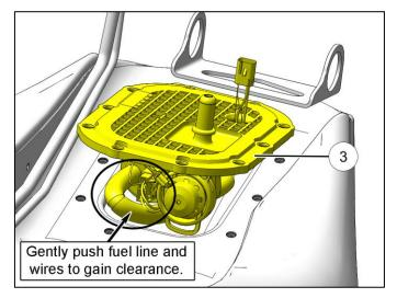
Carefully remove the fuel pump assembly.
