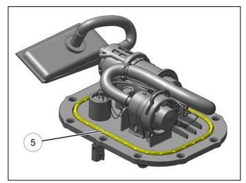
11. Install the new fuel pump assembly making sure the pickup filter lands at the lowest possible point in the tank.
