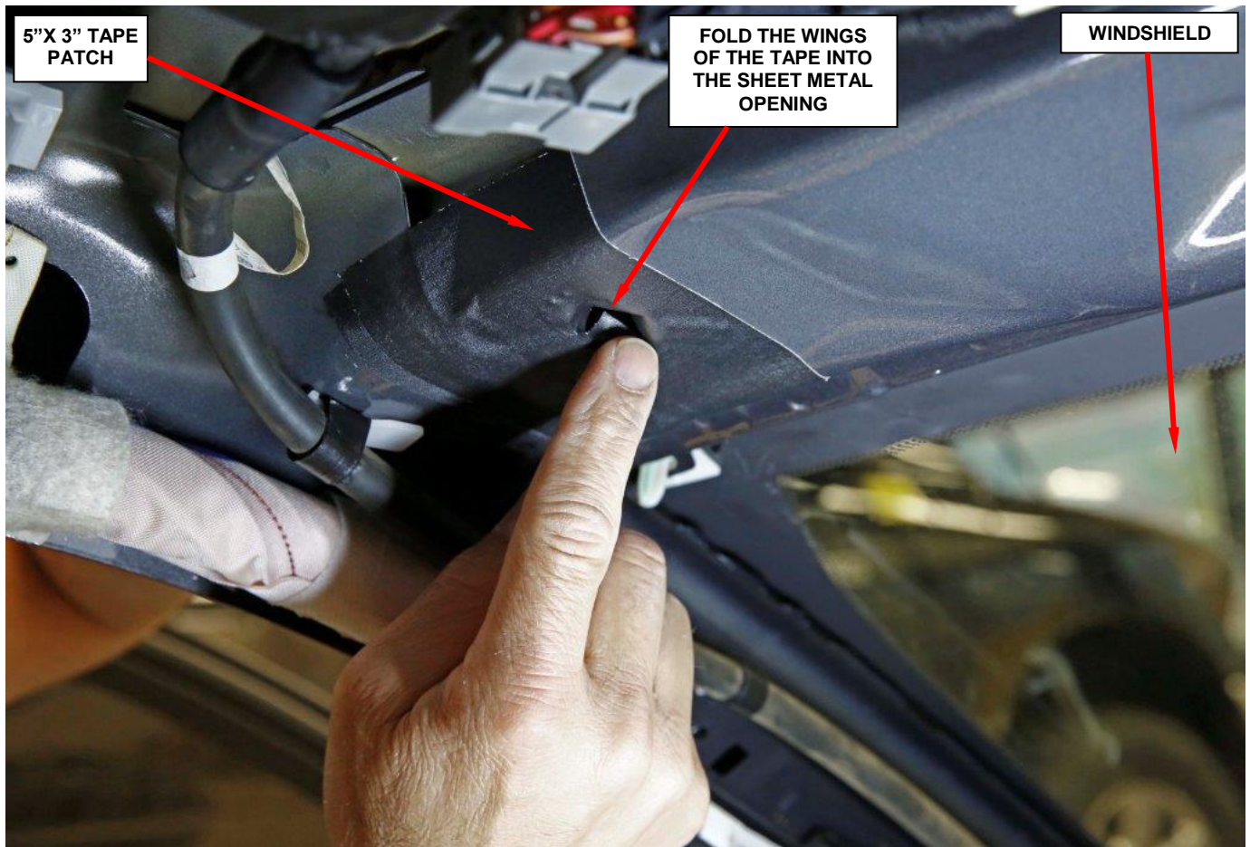
Figure 23 – Fold Tape Wings into the Hole (left side shown)
