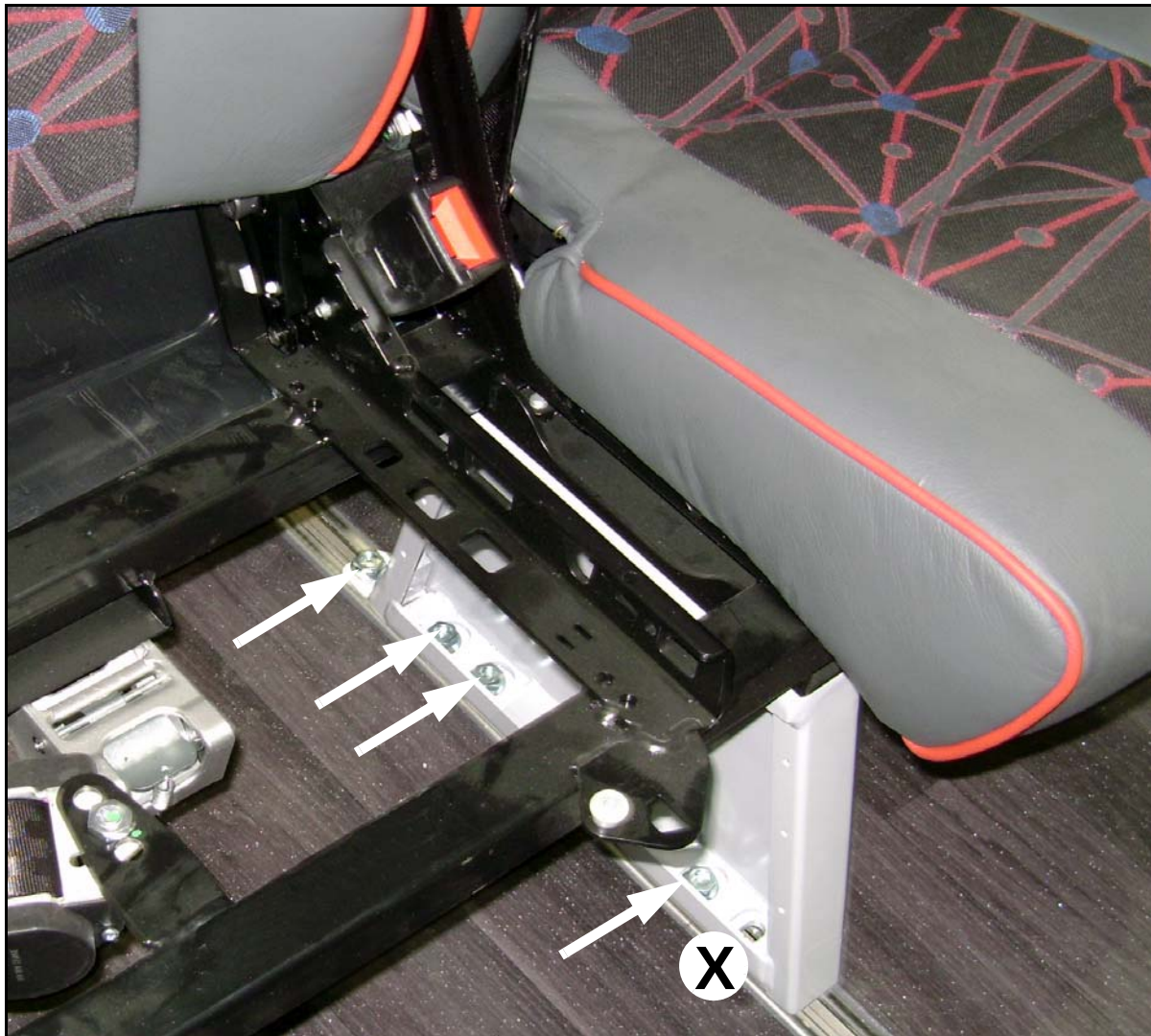
Figure 5. Correct floor track t-bolt location.
