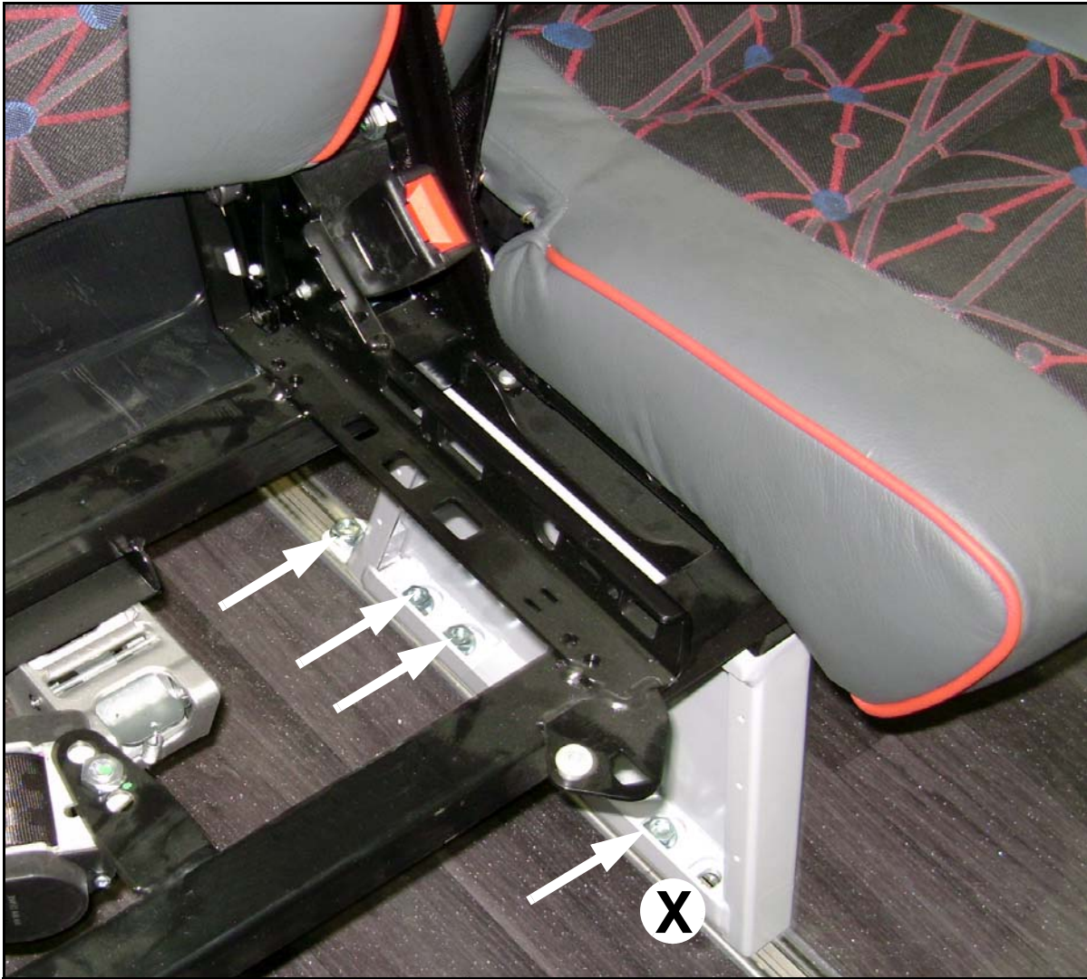
Figure 5. Correct floor track t-bolt location.
