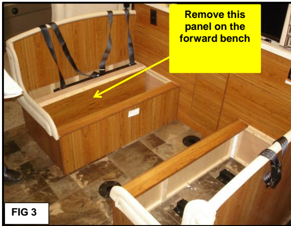
2 Fig 3: Remove the inner panel inside the front bench. Fig 4: Remove 5 screws holding the panel in place, then remove to reveal the seat belt hardware for the forward bench
