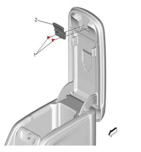
1. Replace the front floor console compartment door latch (2). Refer to *Front Floor Console Compartment Door Latch Replacement* in SI.
