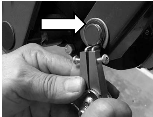
Figure 3. Lower Knuckle Link Arm Snap Ring, Bottom
