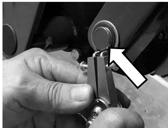
Figure 9. Install Washer and Snap Ring
