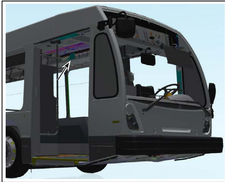
Figure 8 - Smart Sensor (CPU)/APC Analyzer Located in the ITS Tray
