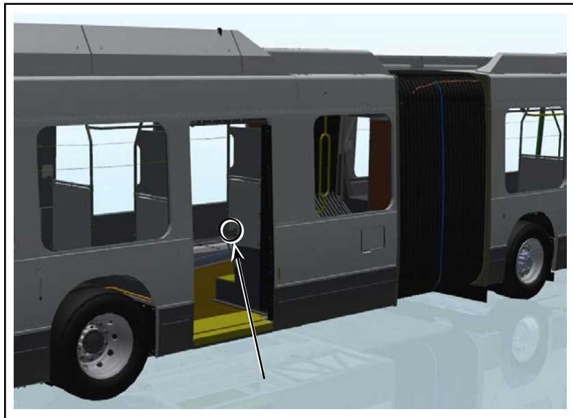
Figure 1 - Passenger Counting Sensor Location
