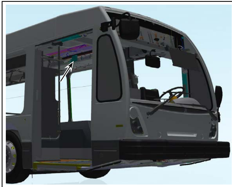
Figure 7 - Smart Sensor (CPU)/APC Analyzer Located in the ITS Tray
