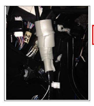
e) Using rubber foam tape insulate both the PCS switch and wires (green and white) to protect them from damage and to prevent rattle noises.
