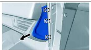
b) Disengage the 3 guides and remove the panel as shown.
