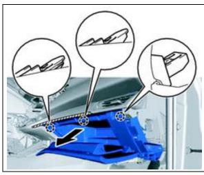
c) Disengage the 3 claws and slowly remove the glove box.
