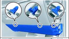
b) Engage the 3 claws to temporarily install the knee airbag.
