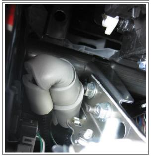
f) After installing the glove box ensure that the relocated PCS switch is still secured and that no wires are contacting the metal brackets located under the dash.
