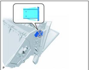
e) Install the switch blank where the PCS switch was previously installed and confirm both claws lock.
