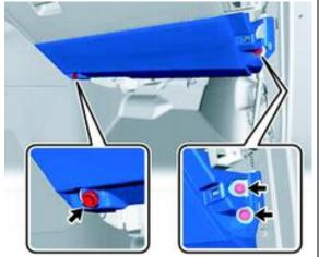
c) Install the 3 bolts and torque to spec.
