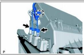
d) Remove the electrical connectors
