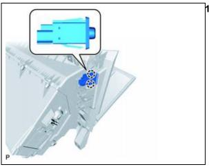
11. REMOVE THE PCS SWITCH FROM THE GLOVE BOX ASSEMBLY
