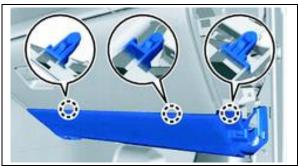
b) Disengage the 3 claws and separate the airbag from the instrument panel.
