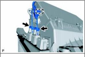
b) Install the connectors as shown..
