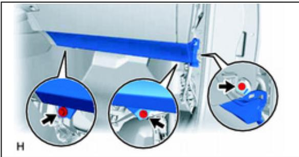
a) Reinstall the 3 bolts and torque to spec.
