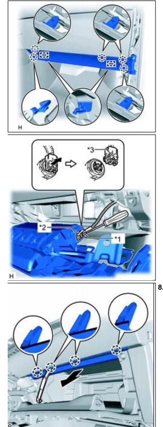
b) Disengage the 5 claws and 2 guides separate the airbag from the instrument panel.
