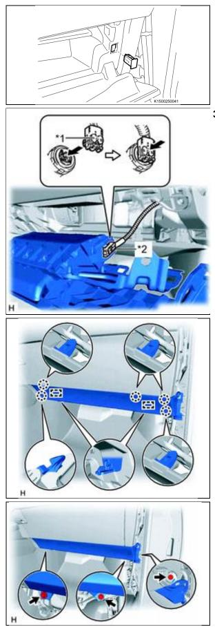
d) Install the switch blank where the PCS switch was previously installed.
