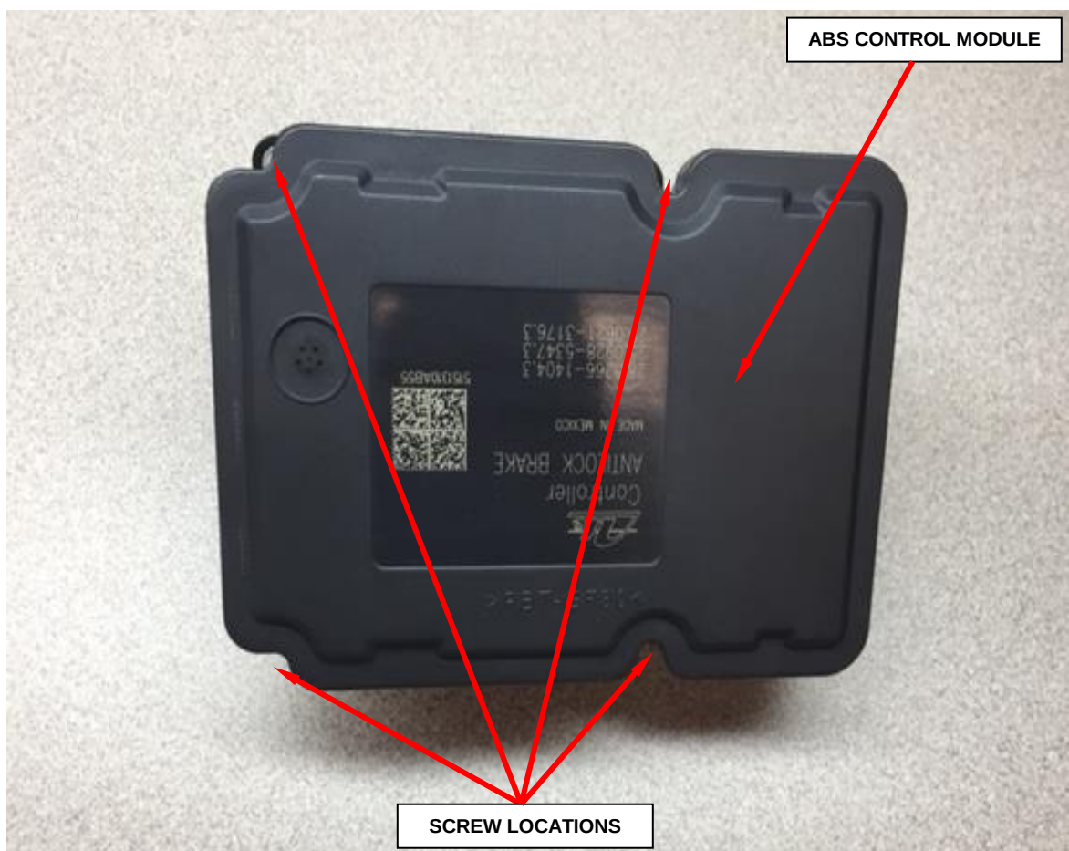
Figure 21 – ABS Control Module
